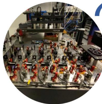
A) Part of current ion-trap quantum computing set-up at PSI
